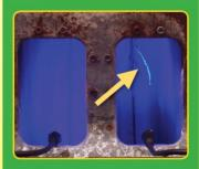
Same view, crack easily observed with the "Crack Finder" penetrant and UV light.
