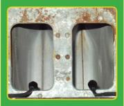
Entrance view of combustion cells of a gas furnace.
